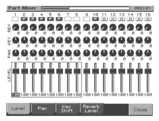
Use [F1]–[F4] to select a parameter, and use the sliders to adjust the values.
